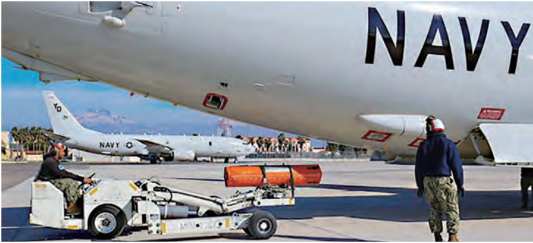
Sailors assigned to Patrol Squadron (VP) 4 load a UNI-PAC II SAR Multi-Mission Air Drop Kit into a P-8A Poseidon multi-mission maritime patrol and reconnaissance aircraft, April 7, 2024.
